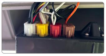
Connect the H-TEC wiring loom plugs into the back of the tachograph in the original order (if your vehicle doesn't have a red or brown plug, please still connect the H-TEC red and brown plugs into the tachograph)
