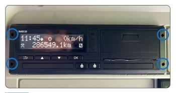
Insert the Tacho removal pins into each side of the tachograph and gently pull the Tachograph out.
