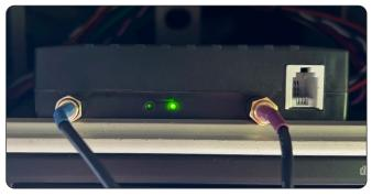
O4 Connect the H-TEC remote download device to the wiring loom. The device should then show some green lights.
